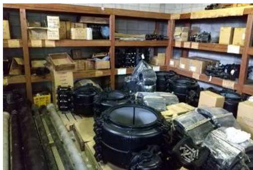
漏水用配管補修材備蓄状況
